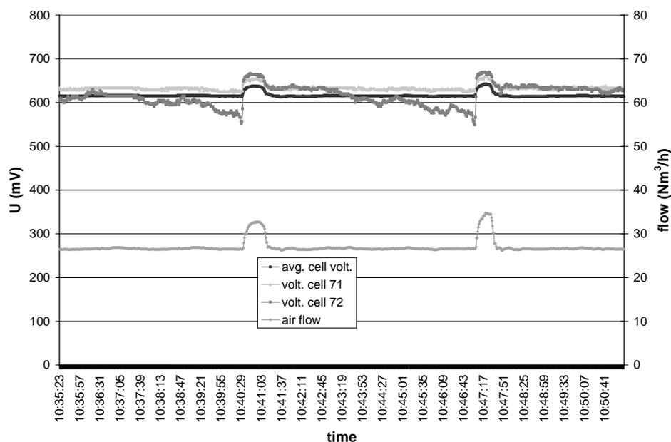
Fig. 5 – Control issue –The time series shows the effectiveness of a gas purge strategy for evacuating water droplets or correcting other gas flow imbalances. It is seen that the voltage of cell 72 decreases steadily. By increasing the air flow rate (represented by the lowest line), the voltage is corrected.
