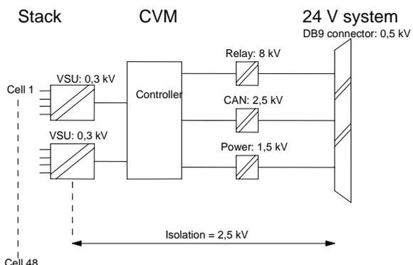
Fig. 1 – The cell voltage monitor lay out with indication of the common mode voltages that can be resisted.
