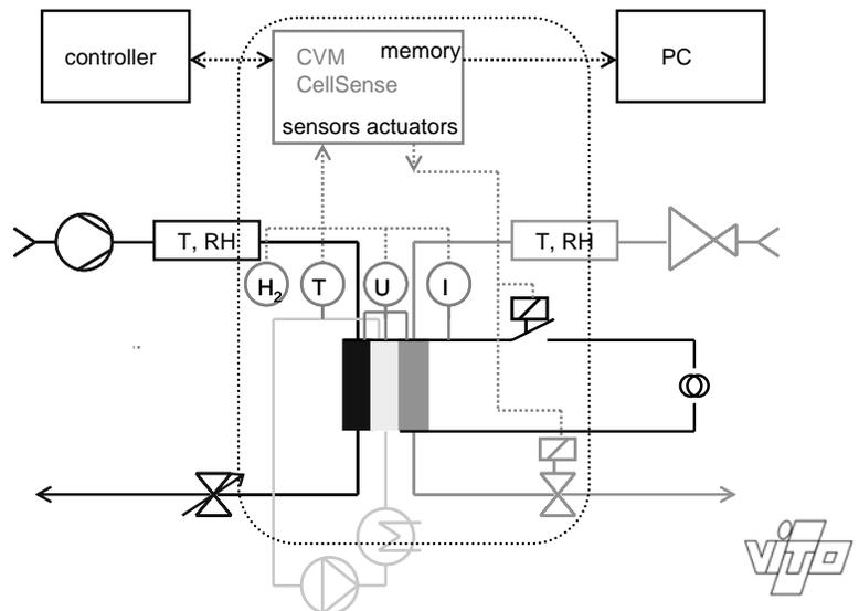
Fig. 9 – Our cell voltage monitor and its role within FC management
