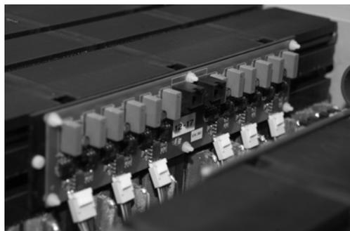
Fig. 2 – A typical arrangement of the cell voltage monitor on a stack.
