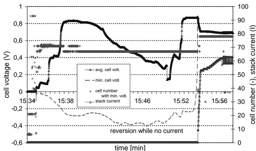
Fig. 3 – Cell voltage reversal at start-up, detected by the cell voltage monitor.
