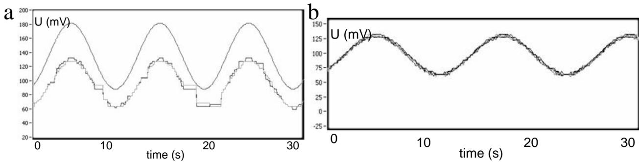
Fig. 8 – Data-transmission of a 0.1 Hz sine waveform by two different methods. (a) By serial RS232. (b) By the CAN, shown for 4 cells. Both figures are screen-dumps during the actual measurement.
