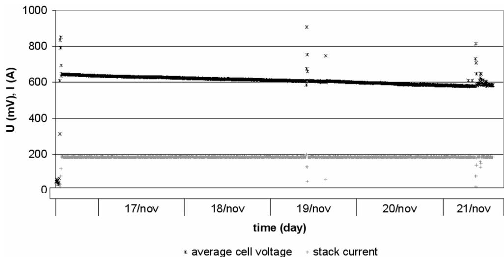
Fig. 7 – Long-term evaluation – Example of stack degradation against time.
